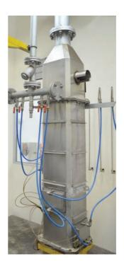
The crude oil from distribution tank is channeled through the reaction chamber installed with ultrasonic transducers. Immediate separation of oil particles will take place and agglomerate to form larger oil globules. Once the treated oil reaches the clarifier, it will be easily recovered.
